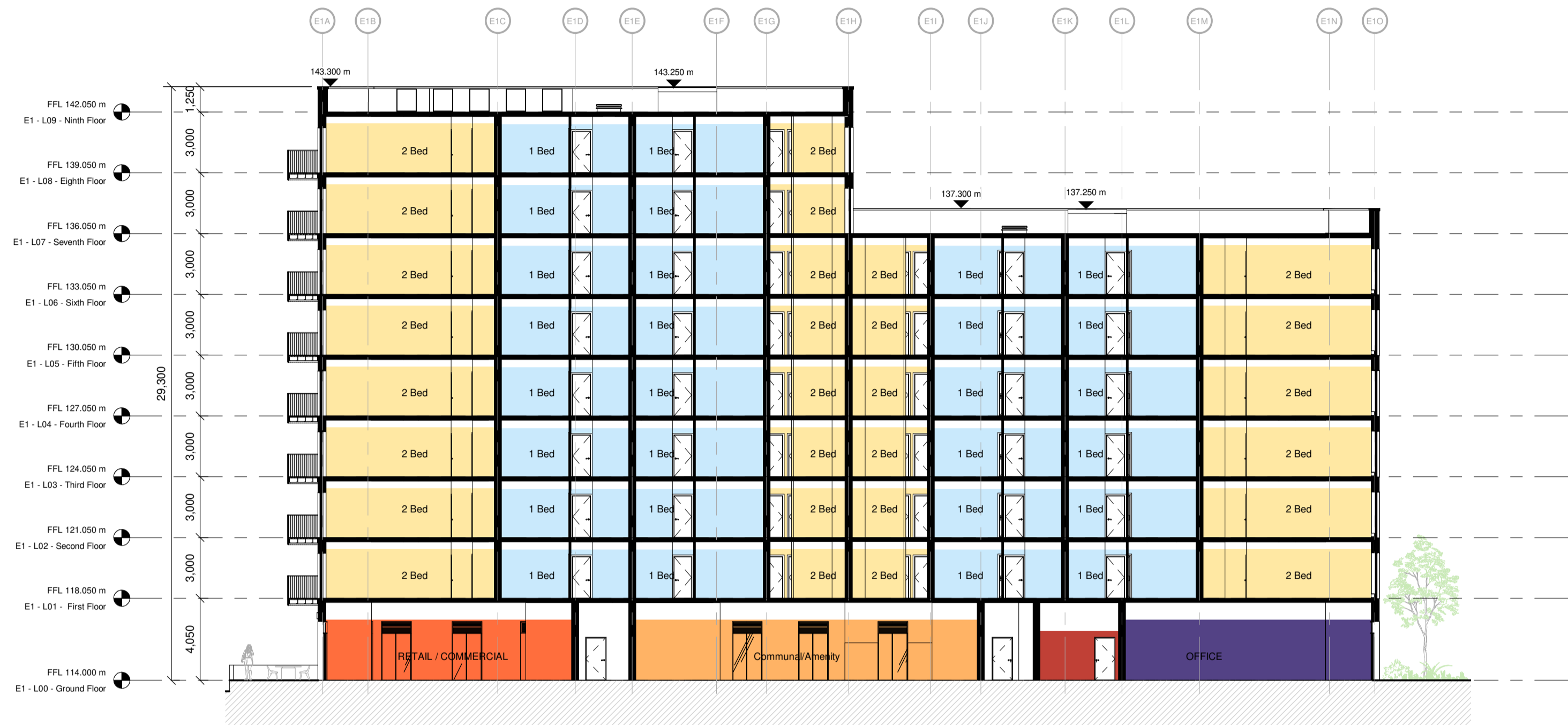
1 PROPOSED SECTION - BLOCK E1 1 : 200
